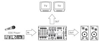
Since the KJ-7808RV has numerous connectivity options, and there exist many variations in user needs, we illustrate a system where all possible connections are used. Note: This is a reference model only. Reference what you need from the diagram. Some connections may not apply for your system.
